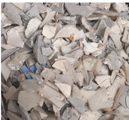
Figure 1: The mixture of plastics (mainly PP and ABS) obtained from postconsumer washing machines (WEEE).
